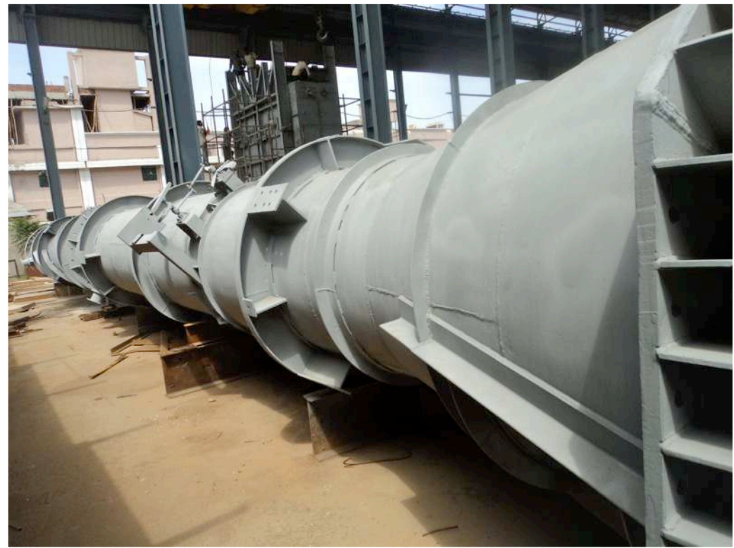
Complete stack after refractory dry-out (with damper installed)
