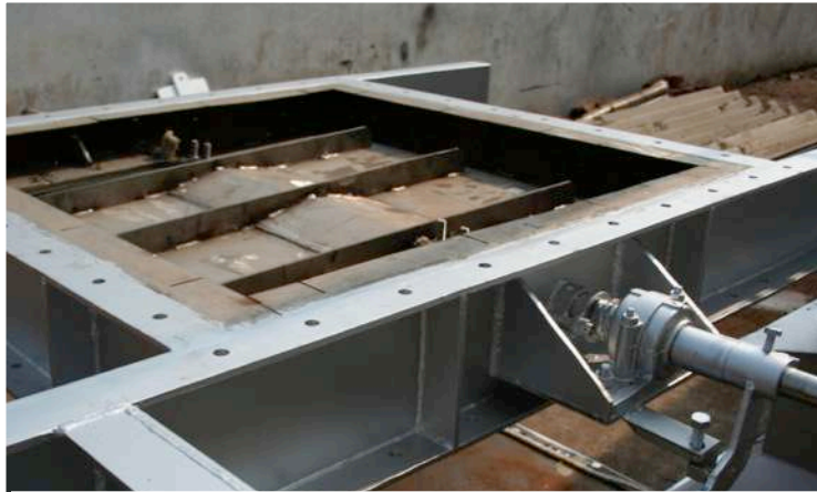
Damper with 99.5% sealing at 900°C design temp – for IOCL, BGR
